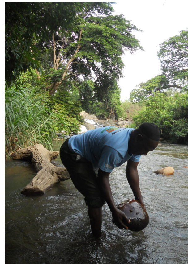
Biomonitoring of streams for water quality and catchment ecosystem health: Lifting a riverbed stone to examine for aquatic macroinvertebrates (insect larvae) underneath.
