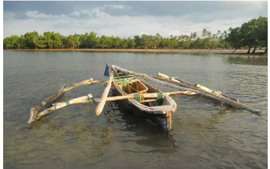
An ngalawa, a sailboat with outriggers, used for fishing in shallow seas, and made entirely out of mangrove poles and wood.
