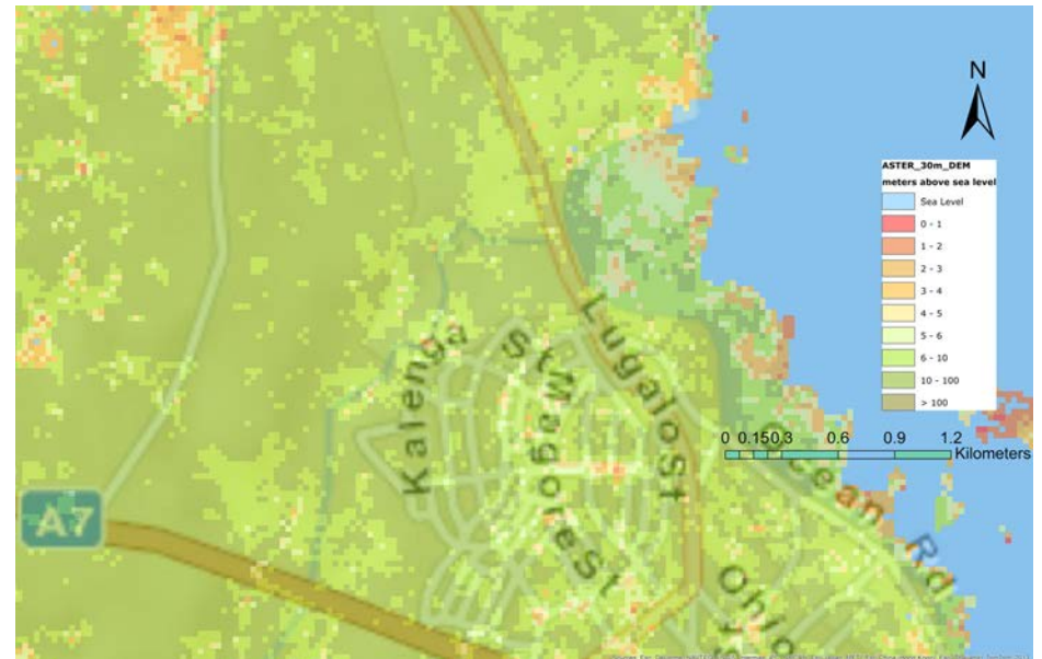
Flooding vulnerability map for downtown Dar es Salaam superimposed on street map. Areas in red have an elevation < 1 m above mean sea level
